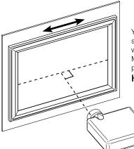
You can slide screen sideways until it lines up with the image horizontally. Make sure projector sits perpendicular to the screen.
